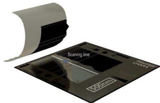
Fig. 3 – Illustration of the removal of the top membrane with an adhesive tape.
