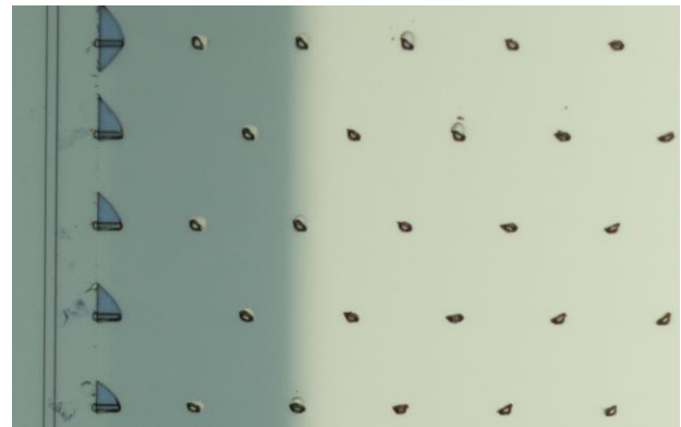
Fig. 4 – A typical microscope image of LHAR test structure showing film penetration (dark area) and distance markers on the chip.
