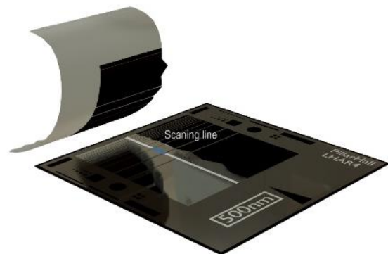
Fig. 3 – Illustration of the removal of the top membrane with an adhesive tape.
