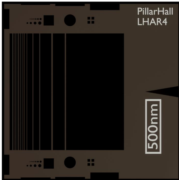
Fig. 1 – Layout of the PillarHall LHAR4 test chip.
