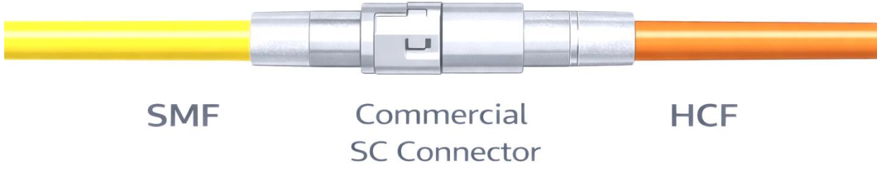
Fig.6. The connection between Standard Single-Mode Fiber (SMF) and Photonic Bandgap Hollow-Core Fiber (HCF) is depicted by this diagram with a commercial SC connector located between the two fibres. The figure shows a high degree of alignment of the fibers by the connector that maintains optimum performance of a low loss transmission. One innovation step in this direction was made by Zhang et al.[29], who created a more complex connector-like interconnection of HCFs, with a record-low IL and at the same time offering pluggability and robustness. The method employed ceramic ferrules (10.5 mm long) that had a funnel shape to ensure that the glue was applied in the area of the end-face and there was no adhesive entering into the HCF core and to give it a greater mechanical stability. To resolve angular misalignment, which is a critical issue of large-MFD HCFs, they utilized connectors that offer auto-collimation to minimize tilt to less than 0.002 rad, which causes minimal loss (<0.07 dB) based on Gaussian mode analysis. The HCF-to-HCF Conjoined-Tube Fibers (CTF) interconnection experimental setup is shown in Fig. 7. The figure depicts the application of a specially designed metallic mating sleeve with a 3X4 slot layout, which allows it to be rotated by 30°. This modification makes it possible to reduce transverse offsets, which are due to the non-concentricity of the cores and offsets at the ferrule. The outcome indicates that there is an IL of minimum 0.13 dB at 1550 nm and the standard deviation of 0.03 dB, over 10 plug-unplug trials. This is the highest record ever made for fusion splicing (0.16 dB) and is close to the theoretical mismatch limit (0.074 dB). Moreover, mode-field adaptation is necessary to overcome the MFD difference (10.4 \mu\text{m} in the case of SMF and 27.9 \mu\text{m} in case of CTF) in the case of HCF-to-SMF (SMF-28) interconnections. Two of the adapters tested by Zhang et al. were the Graded-Index Multimode Fiber (GIF) and Thermally Expanded Core (TEC) SMF. The TEC-based adapter was also superior, with better mode-field matching (its circular mode profile) and with an IL of 0.10 dB at 1489 nm (0.135 dB at 1550 nm), the lowest recorded of any HCF-SMF joint, only 0.03 dB above the theoretical limit based on MFD mismatch. It is an innovative connector-based system that provides a strong connection between HCFs and SMFs at low loss and high efficiency, and is optimally applicable to high-rate communication systems, quantum networks, and other photonic systems [29].
