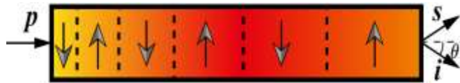
77 Figure 1. Scheme of noncollinear SPDC in a chirped QPM crystal. The directions of arrows represent polarized axis for the QPM PPLN or 78 PPKTP crystals. p, s, i represent the pump, signal and idler lights.
