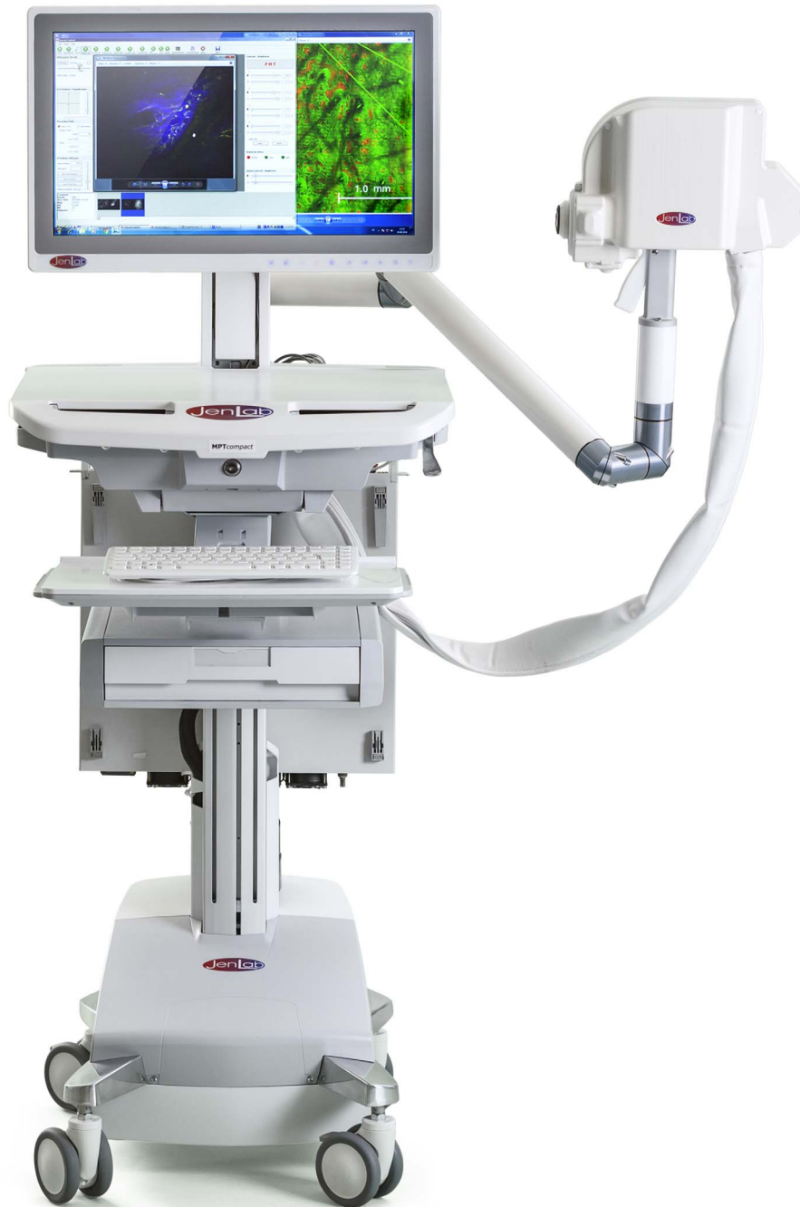
Fig. 4. The novel multimodal multiphoton tomograph MPT compact . The ultracompact fiber femtosecond laser is positioned inside the measurement head. A chiller and an optical arm are no longer required. The tomograph measures (i) 780 nm-excited autofluorescence of intratissue melanin, keratin, elastin, and the coenzymes NADH and flavins by time-correlated single photon counting, (ii) SHG at 390 nm from the collagen network, and (iii) confocal reflectance of the 780nm beam e.g., from the cell membranes. Furthermore, white-light images are provided for dermoscopy and laser beam location.
