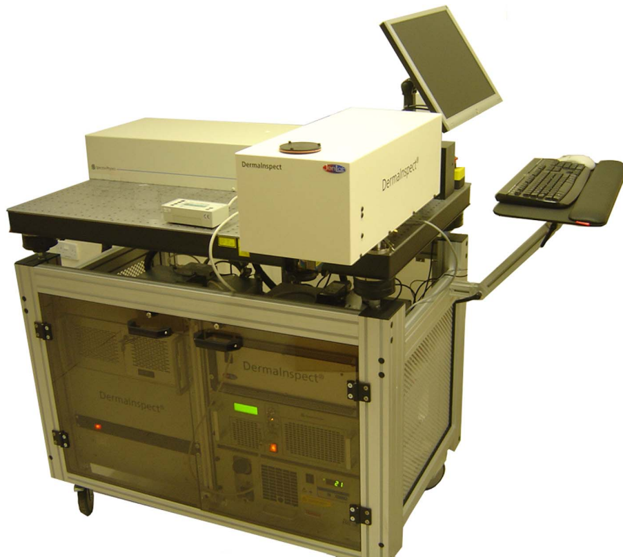
Fig. 2. The commercial multiphoton tomograph DermaInspect (laser class 1M) for high-resolution tissue imaging with a tunable near infrared 80 MHz femtosecond laser and time-resolved single photon counting (TCSPC) received the certificate of conformity as a class 2a medical device in 2004.
