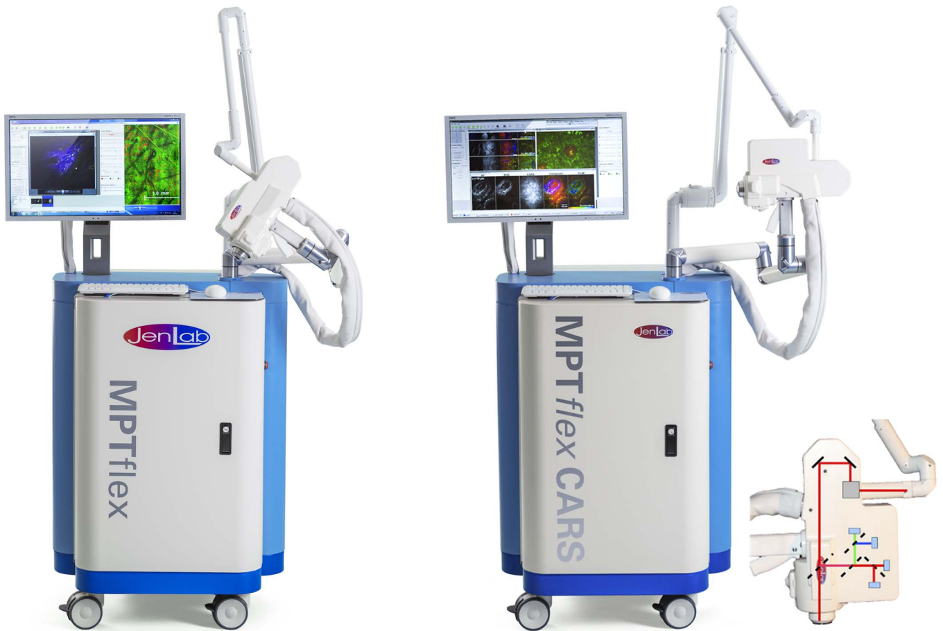
Fig. 3. The second generation of multiphoton tomographs MPTflex is easy to move and possesses an optical arm with a 360° measurement head. The MPTflex received the certificate of conformity as a medical device in 2010. Left: “conventional” MPTflex with two PMT detectors. Right: Two-beam multiphoton tomograph MPTflex-CARS with four PMT detectors to measure simultaneously time-resolved autofluorescence, SHG, and Raman signals of lipids/water.
