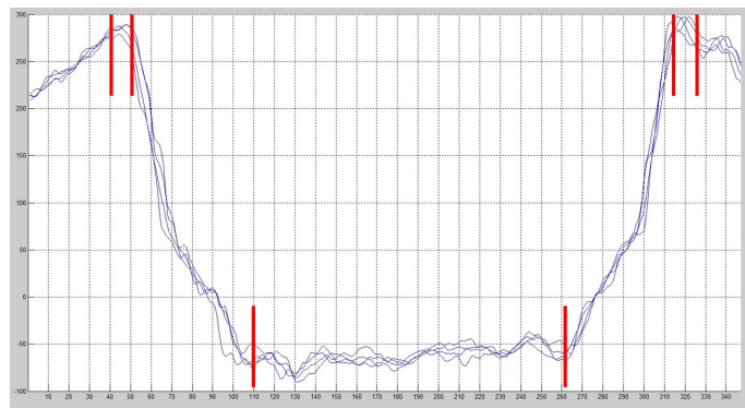
FIG. 3 MATLAB experiments analysis. Showing in the X-axis every 100 nanometres the material removal depth. Showing in the Y-axis every 10 pixels the distance of the cross sectional line.
