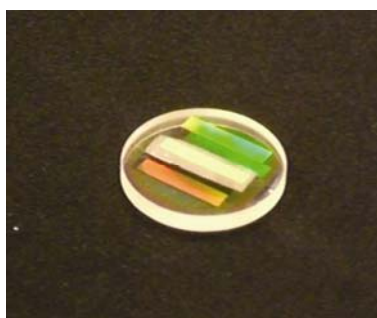
Fig. 7 Picture of a monolithic phase mask made on a 1 inch substrate. Gratings G_2 are visible at both sides of grating G_1 , covered by an aluminium layer.
